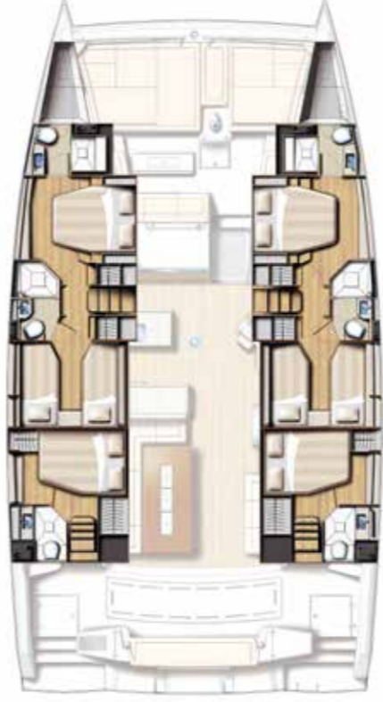
6 CABINS / 6 BATHS VERSION (4 doubles + 2 central twins) Version 6 cabines (4 doubles + 2 twins centrales) / 6 sdb
